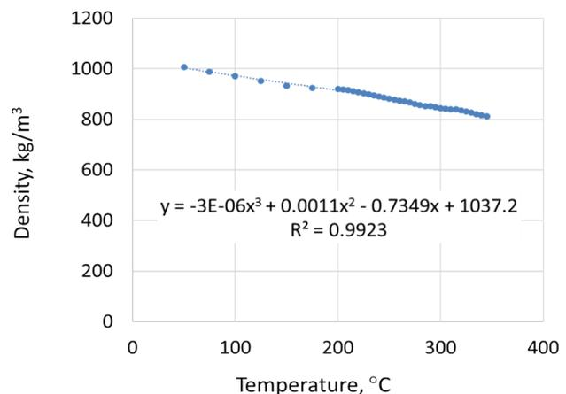
**Figure7.** Curve fitting for experimentally measured values of density of oil versus temperatures
