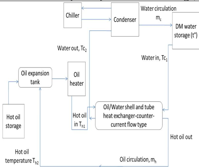
**Figure 3.** Schematic of test setup for evaluation of heat transfer fluid
