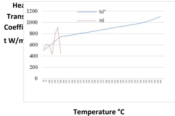
**Figure 10.**The empirical and calculated convective heat transfer coefficients,  $hi''$  and  $hi$ , shown from 50°C up to 200°C and 400°C, respectively
