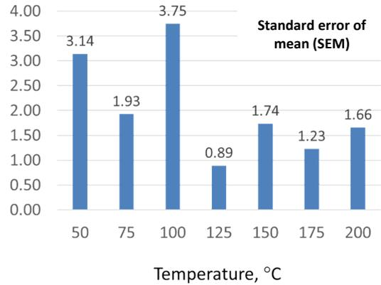
Figure I.2. Standard Error of Mean (SEM) Values for  $h_i$  obtained using the Wilson Plot Technique
