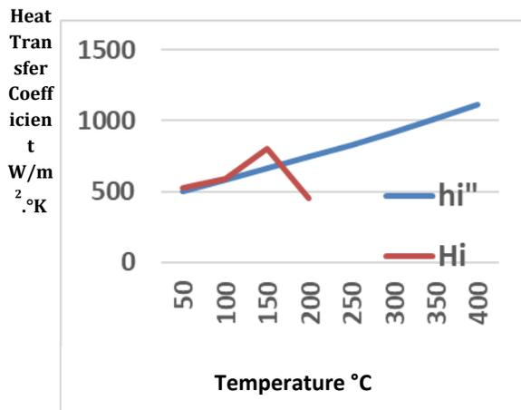
**Figure 11.** Convective heat transfer coefficients plotted at uniform temperature intervals of  $25^{\circ}\text{C}$  for entire operational temperature range of solar grade synthetic oil
