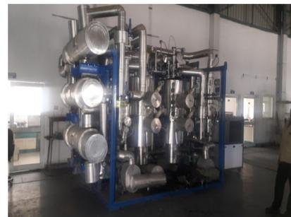
**Figure 2.**Photograph of the test setup for evaluation of heat transfer fluid
