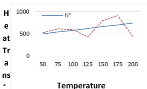
**Figure 6.** Comparison of Convective heat transfer coefficients  $h_i''$  and  $H_i$  up to experimentally measured temperatures of 200°C.
