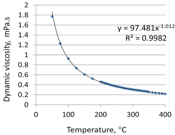
**Figure 8.**Curve fitting for experimentally measured values of dynamic viscosity of oil versus temperatures
