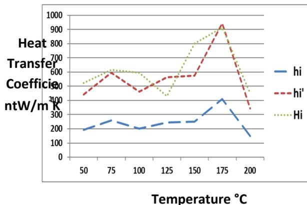
**Figure 5.** Superimposition of the heat transfer coefficient curve obtained through Wilson plot onto that obtained from calculation using classical thermal resistance equation
