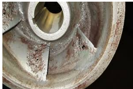
Fig. 1. Damaged centrifugal pump impellers due to cavitation
